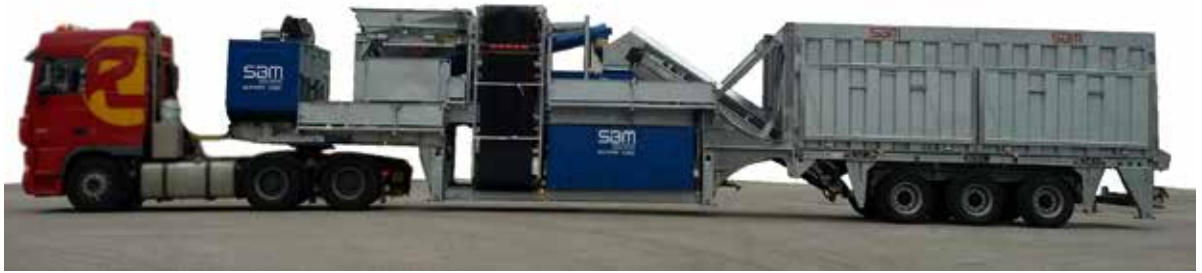
Road-transport capable EUROMIX 400 SM C inline plant for recycling concrete
